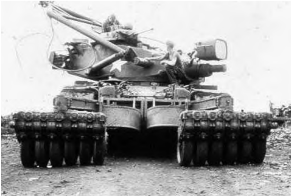
Rollers placed in front of M48 tanks and this combat engineer vehicle expedited clearing roads of mines.
